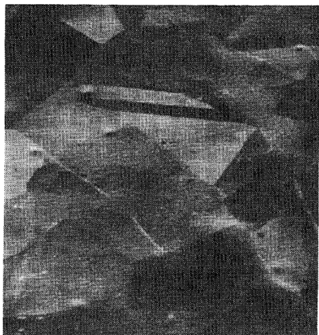
Fig. 2. SEM image of a Cu-0.28 wt% Al alloy sample (absorbed current mode).
